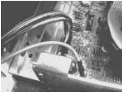
Attach the protective earth, green / yellow, ground wire.
