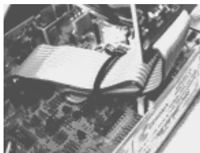
Plug in video board. Fold video flat cable to avoid contacting the metal frame. Secure fold with a wire tie.
